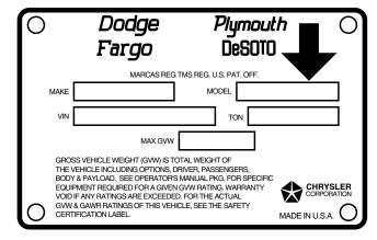
On 1967-81 Dodge Trucks the engine model designation consists of the cubic inch displacement followed by a dash number. In many cases, the correct dash number must be known to determine the correct spark plugs to be used. The correct dash number is determined by first locating the Vehicle Identification Plate (rear face of driver's door or driver's side latch post).
