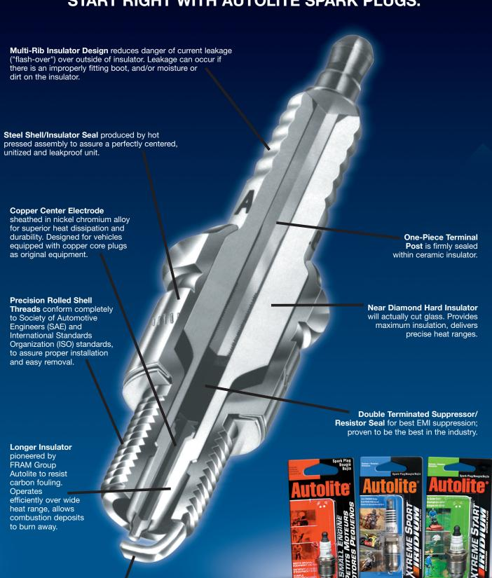
Ground Electrode nickel chromium alloy resists gap growth and maintains precise spark gap longer.
